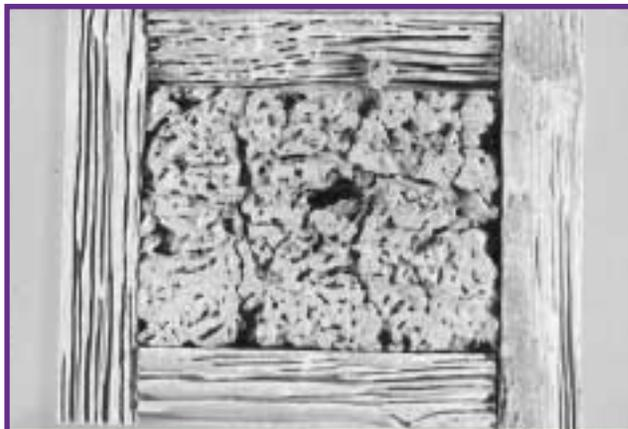
**Wood damaged by the Formosan subterranean termite is surrounding carton material produced by the termites.**
