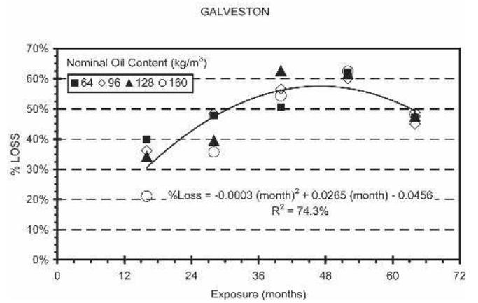
Figure 6. — Depletion rates by oil content for the above-ground zone in two test plots.
