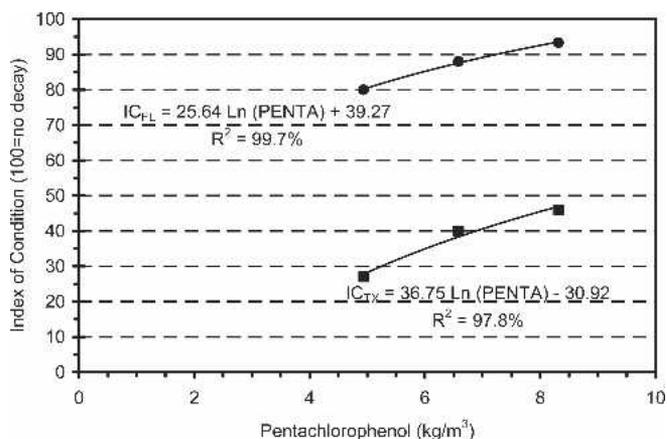
Figure 1. — Dose-response curves for matched stakes treated with penta after 5 years of exposure in Galveston (TX) and Gainesville (FL).
