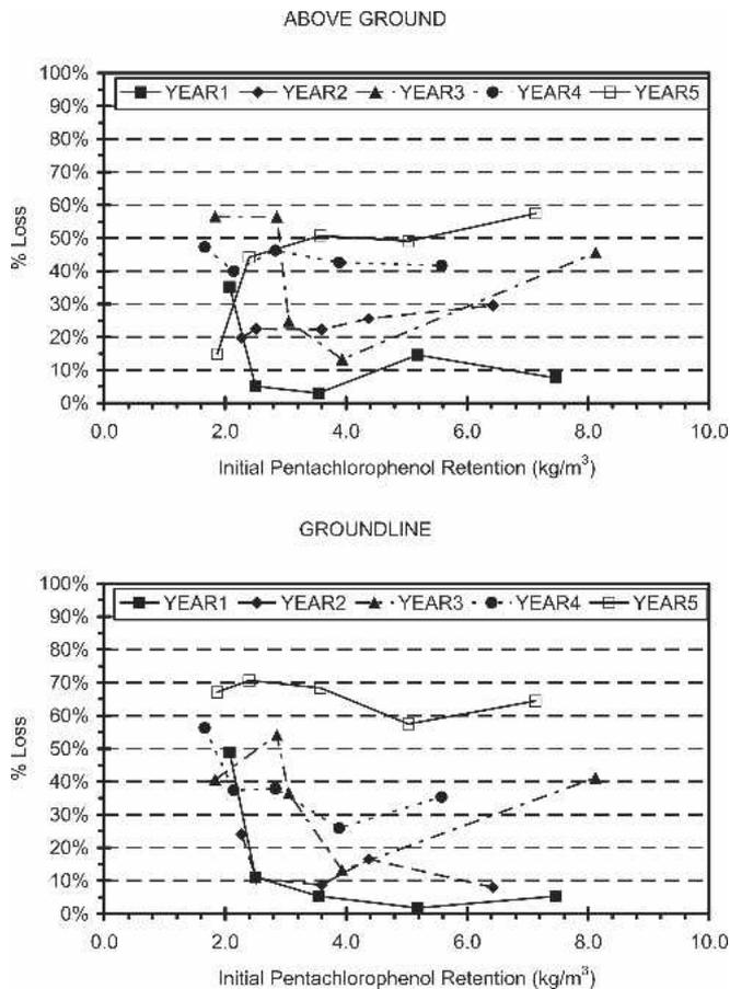
Figure 4. — An example of the data scatter by year for aboveground (upper) and groundline (lower) preservative loss vs. initial preservative retention for the 160 kg/m<sup>3</sup> oil content stakes in the Harrison Forest test plot.
