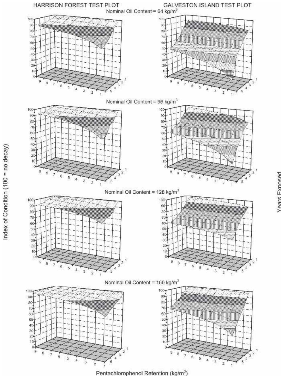
Figure 2. — Dose-response curves by year at four nominal oil contents for stakes treated with penta in AWP A P9 type A solvent and exposed at the Harrison Forest (left) and Galveston Island (right) test sites.
