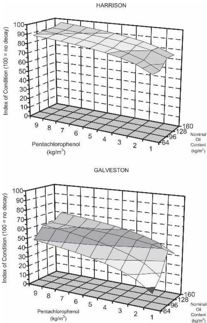
Figure 3. — Effect of oil content on the performance of penta in P9A oil after 5 years of exposure in the Harrison Forest (upper) and Galveston Island (lower) test plots.
