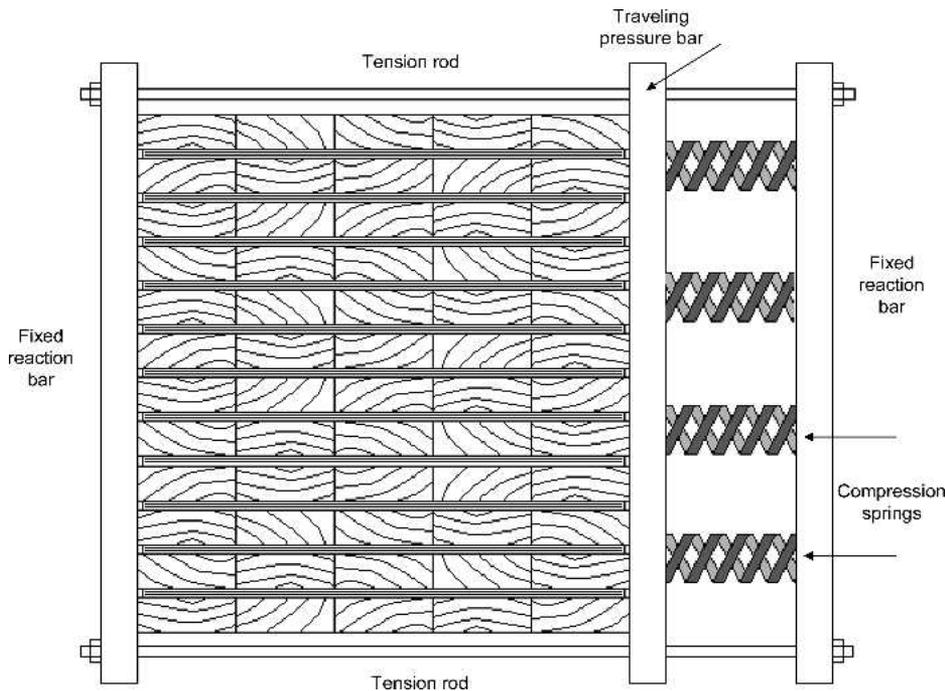
Figure 1. — Section view of one of the three restraint device clamps.
