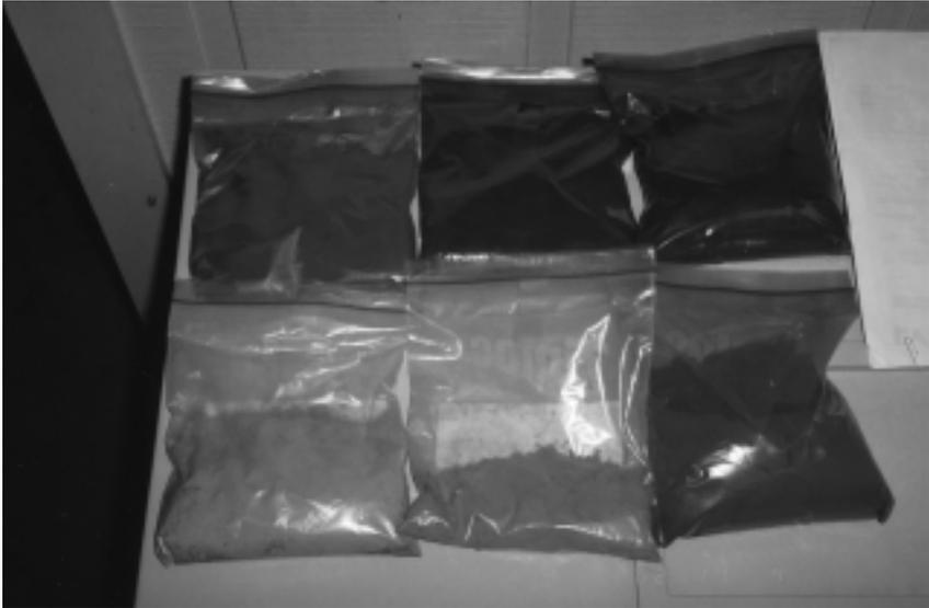
Figure 1. — Appearance of six filler flours for bonding plywood in PF resin-adhesives. Top row, left to right: 65 percent E. walnut shell flour/35 percent oat hull furfural residue; oat hull furfural residue; Asian furfural residue. Bottom row, left to right: E. walnut shell flour; pecan shell flour; alder bark flour.
