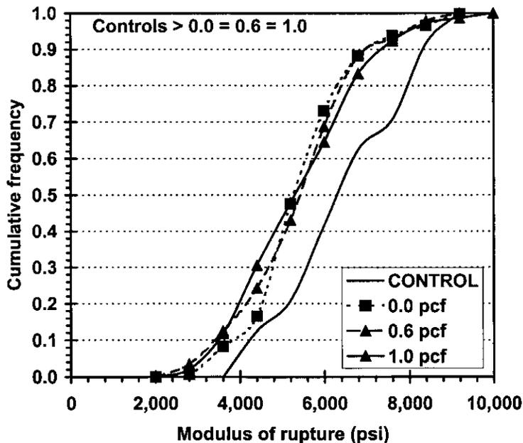
Figure 3. — Effect of retention on modulus of rupture distributions.
