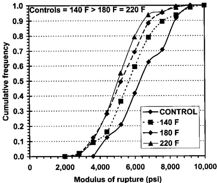
Figure 4. — Effect of temperature on modulus of rupture distributions.
