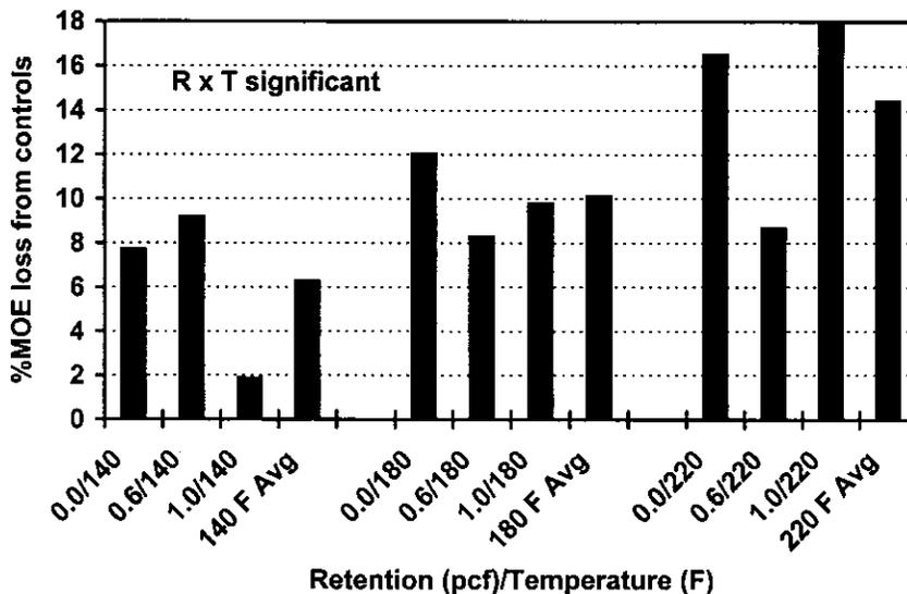
Figure 2. — Percent loss in MOE by retention/redrying temperature.
