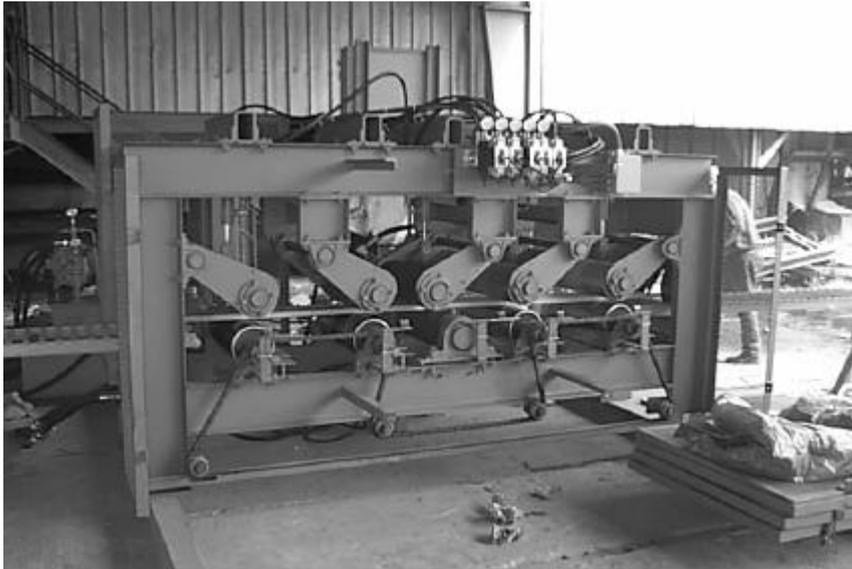
**Figure 3.** Corley commercial prototype TASK Process machine being used to mechanically stress lumber with compression and/or vibration.
