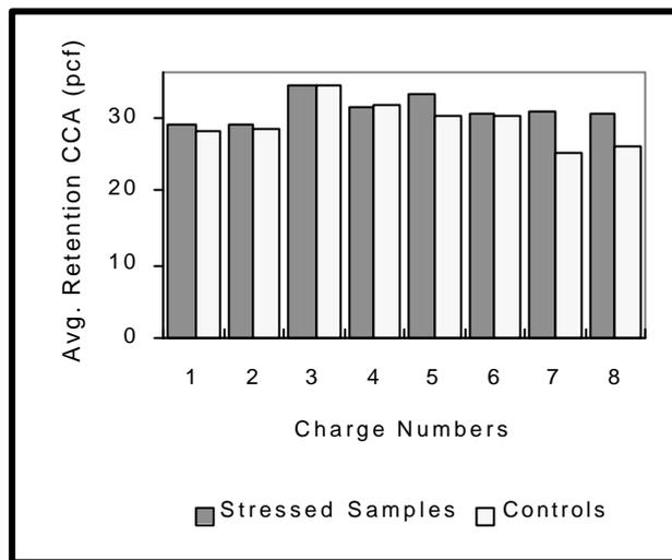
**Figure 2.** Samples from initial studies at MSU had increased retention of preservative in the mechanically stressed pieces.
