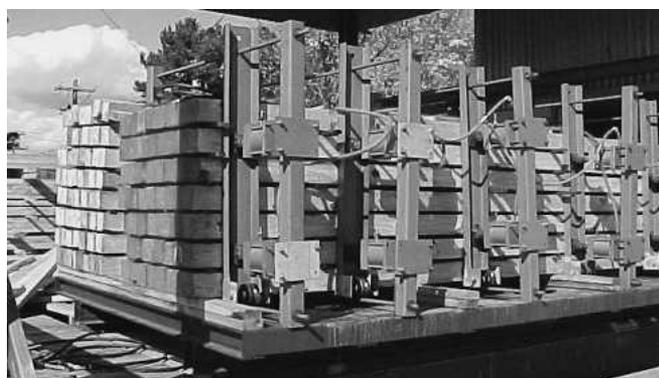
Figure 2. — Photograph of the two matched lumber packages immediately following initial kiln-drying. The depressurized restraint device is still attached to the right-hand package.
