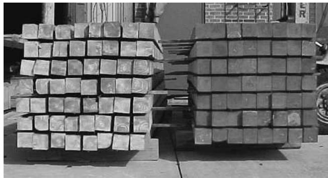
Figure 3. — Photograph of the two matched lumber packages immediately following initial kiln-drying. With the restraint device removed, pieces in the right-hand package appear less warped.
