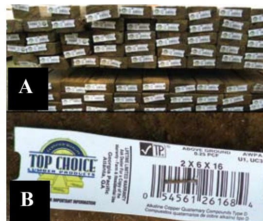
Figure 8.A.) Replacement materials for the deck in Fig. 13. The tags on the ends of the new decking (B) indicate that the lumber was treated with alkaline copper quaternary (ACQ) compounds, Type D by Georgia Pacific to a retention of 0.25 pounds per cubic foot and is to be used in AWPA use categories U1, UC3B (exterior construction, above ground) as defined in the AWPA Book of Standards. Each board was stamped on one face showing that the wood was inspected by an SPIB inspector who determined its grade to be No.2.
